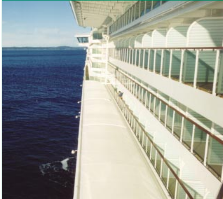
The clean and uninterrupted lines of the sandwich composite panelling.
