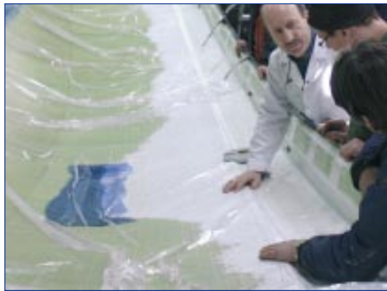
A demonstration of the DIAB Core Infusion Method.
